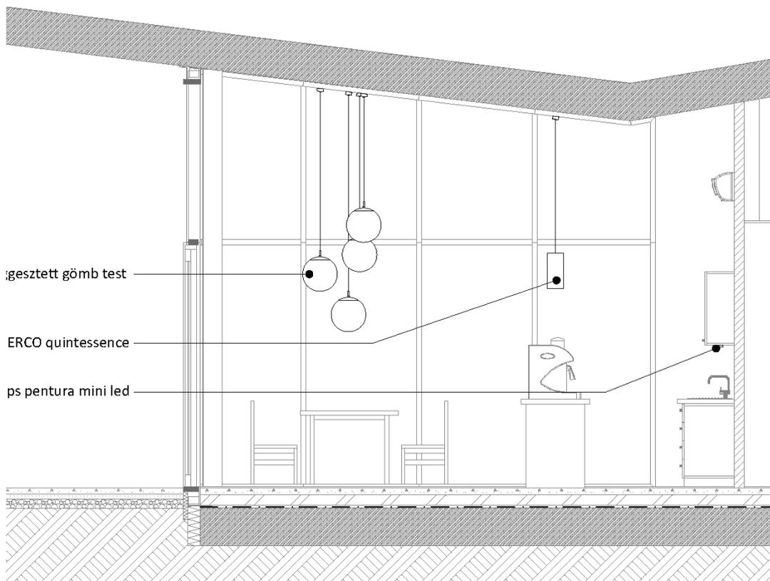
**Calculations using manufacturer specific luminaires and light sources**
