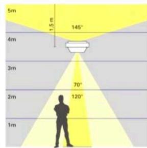
Light cone adjustment with focusing the down/light from 60° to 100°.
