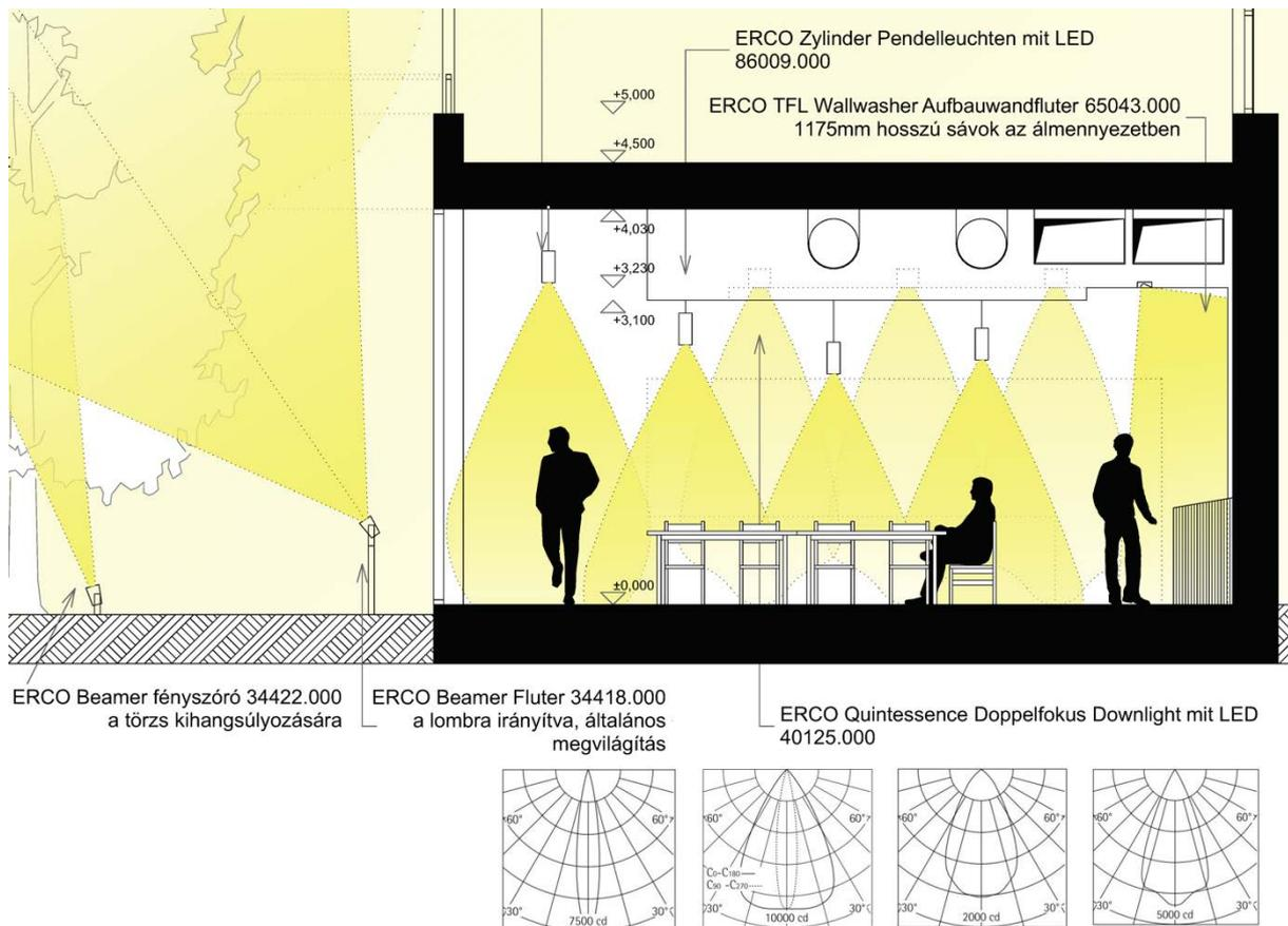
Artificial light source distribution diagrams and lamp distribution indicated on a building section (Borbála Birges)
