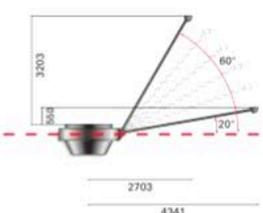
Inclination of the support rods: 20° angle up to a 60° angle.
