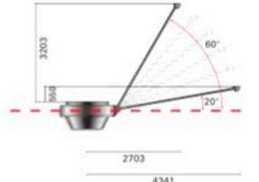
Inclination of the support rods: 20° angle up to a 60° angle.
