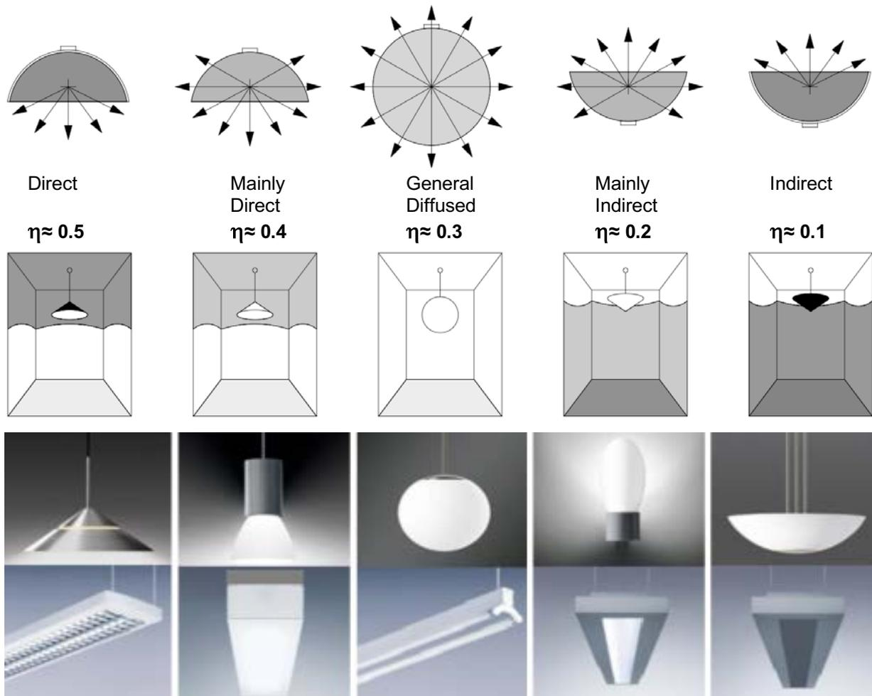
Light distribution and efficiency of luminaires
