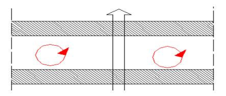
Maximum temperature difference is given for an inner surface and ambient temperature of a composite wall construction. This is due to surface condensation and mould growth problem.
