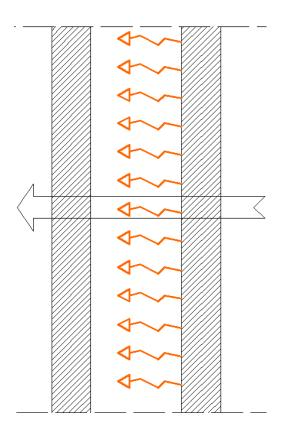
Also a rate of heat transfer trough an air gap depends on the direction of heat flow in horizontal cases.
