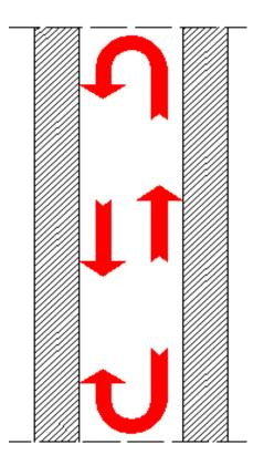
There is a **radiant heat exchange** between the opposite boundary surfaces.
