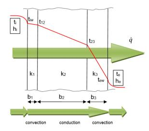
$$R = R_i + R_p + R_{brick} + R_p + R_e = \frac{1}{h_i} + \frac{b_{plaster}}{k_{plaster}} + \frac{b_{brick}}{k_{brick}} + \frac{b_{plaster}}{k_{plaster}} + \frac{1}{h_e}$$
