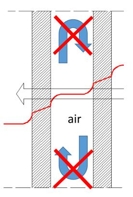
Due to the **density difference** <u>natural air</u> <u>circulation</u> accompanied with convective heat transfer develops in vertical air gaps and depending on the direction of the heat flow in horizontal ones.
