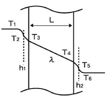
We are really concerned with the rate of heat transfer between the two sides of the composite slab rather than the process between surfaces. It is convenient to define an overall heat transfer coefficient (U-value), given by:
