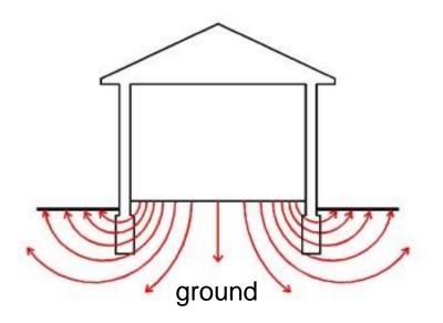
Ground and footing losses are calculated with **linear heat transfer coefficients** too, along the perimeter of the building.
