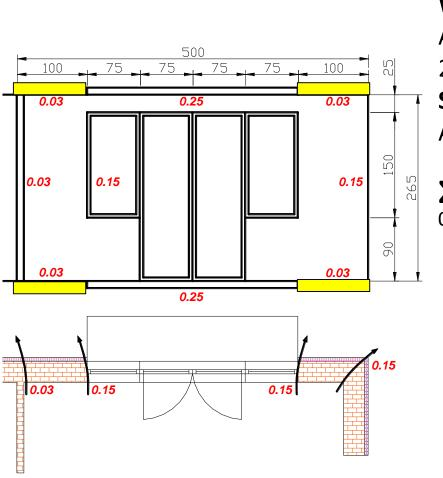
**Total surface:** A=5.2.65=13.25m2 Window surface: A<sub>w</sub>=2.0.75.1.5+1.5.2.4m= 2.25+3.6=5.85m2 Surface of the brick wall: A<sub>wa</sub>=A-Aw=13.25-5.85=7.4m2  $\nabla \Psi \cdot \mathbf{I} =$  $0.15 \cdot (3 + 1.5 + 1.5 + 2 \cdot 0.75 + 2 \cdot 0.9)$ =1.395W/K window  $0.15 \cdot 2.65$ =0.398W/K corner  $0.25 \cdot (3+3)$ =1.500W/K balcony =0.120W/K ring beam  $0.03 \cdot (2+2)$ 0.03 · 2.65 =0.080W/K partition Sum: =3.493W/K
